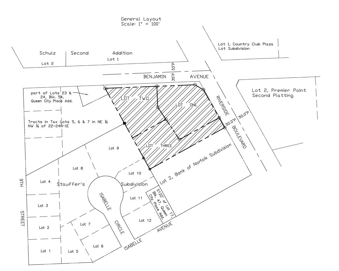
1) Bearings are based on Grid North (US/NAD83/NE Datum) based on direct observation using G.P.S. equipment on the HPRTK Network.
